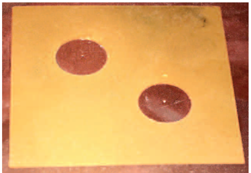
Figure 2 - Low-Flow Test Coupon
